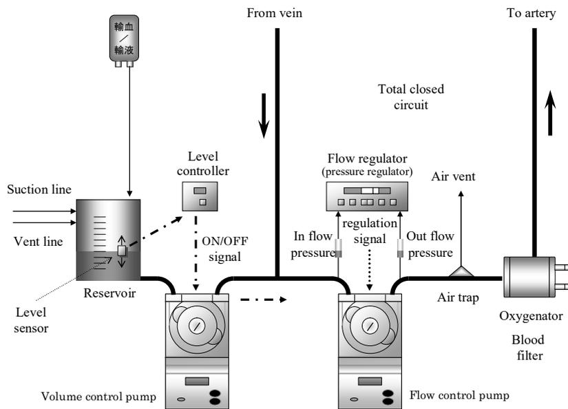
Automatic volume control (AVC) & Automatic flow control (AFC)
